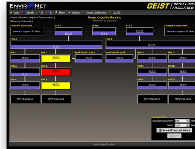
Power Capacity Planning View
